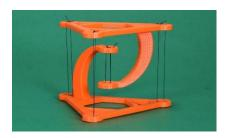
However, seemingly independent parts can be arranged in a balance of tension and compression, by means of cables or tendons. READ MORE
